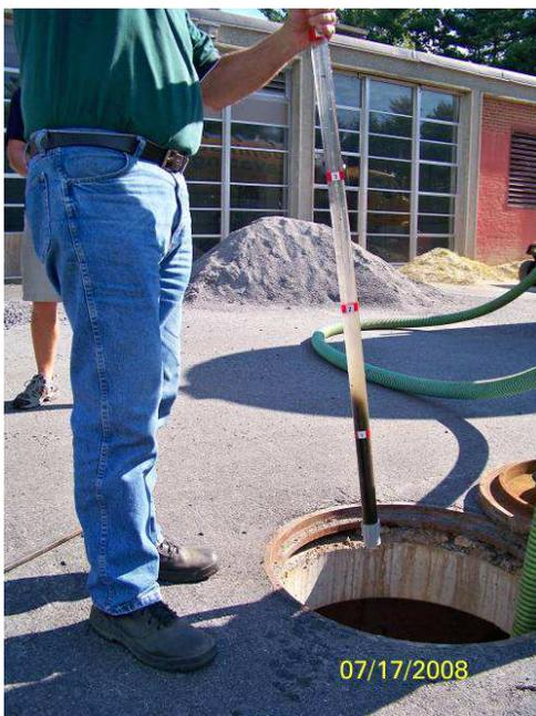
The depth of sediment and oil can be measured from the surface by using a sediment probe or dipstick tube equipped with a ball check valve and inserted through the Jellyfish Filter's maintenance access wall opening. The large opening provides convenient access for inspection and vacuum removal of water and pollutants.
