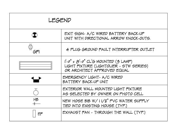
ELECTRICAL CONTENTS GFI OULTETS EXIT LIGHTS EMERGENCY LIGHT I EXTERIOR LIGHTS 2 EXHAUST FAN
