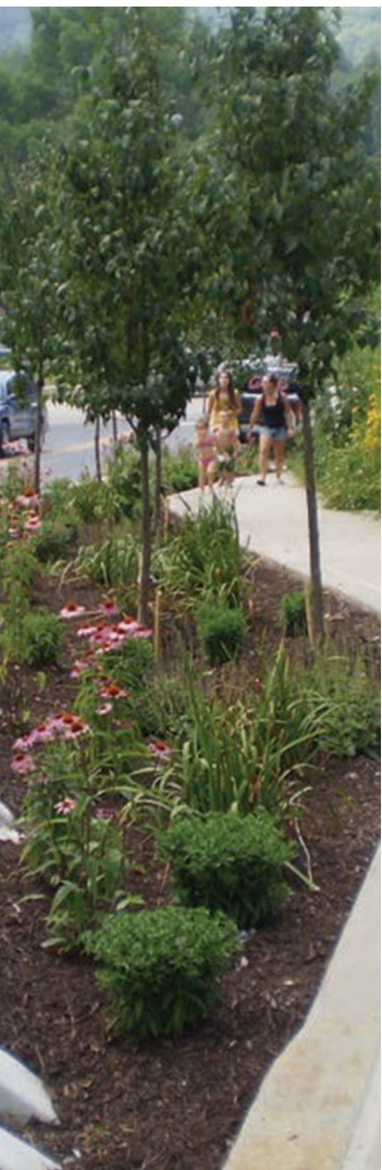
Bioswales improve on-site stormwater management and are an interesting landscape element.
